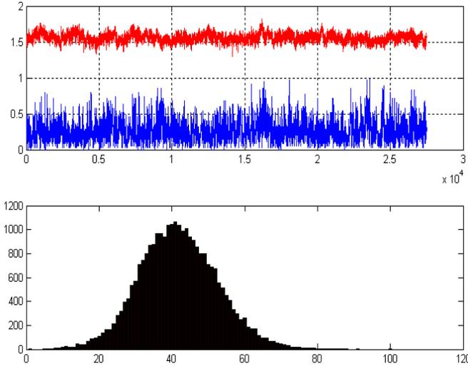
Fig. 6. Knock Airport (12/11/2003-1/1/2005) for hourly (averaged) sampled data. Above: Normalised wind velocity data  $v(t)$  (blue) and the Lévy index  $\gamma(t)$  (red) for a look-back moving window of 1024 elements. Below: 100-bin histogram of  $\gamma(t)$ .
