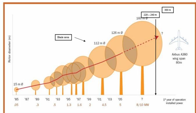
Fig. 1. Schematic diagram of the increasing size in wind turbine blade area (rotor diameter) from 1985 onward required to provide larger power yields according to the Betz law in which the power from a wind turbine is proportional to the blade area (Source: Jos Beurskens ECN).
