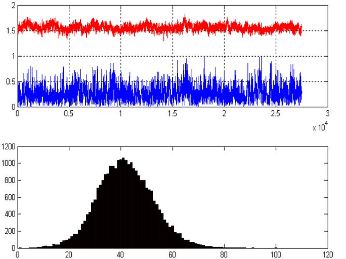
Fig. 5. Cork Airport (12/11/2003-1/1/2007) for hourly (averaged) sampled data. Above: Normalised wind velocity data  $v(t)$  (blue) and the Lévy index  $\gamma(t)$  (red) for a look-back moving window of 1024 elements. Below: 100-bin histogram of  $\gamma(t)$ .
