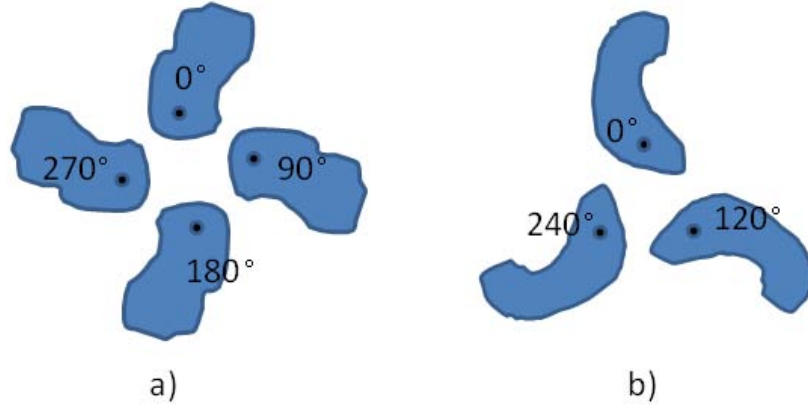
Figure 2.5. Visualisation of sequentially rotated array with three (a) and four (b) elements. The numbers indicate phase shift, at which each element is fed. Generated wave will be RHCP into the page and LHCP out of it.
