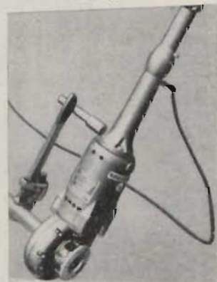
AMAZ-O-THREAD. So light it can be carried with one hand. Threads up to 2" i.d. in less than 30 seconds.
