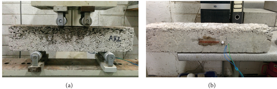
FIGURE 1: Flexural beam tests (a) during test and (b) with a strain gauge attached.
