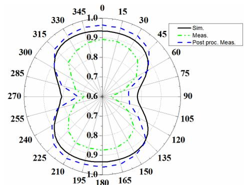
Figure 4: Simulated, measured and post processed FF.
