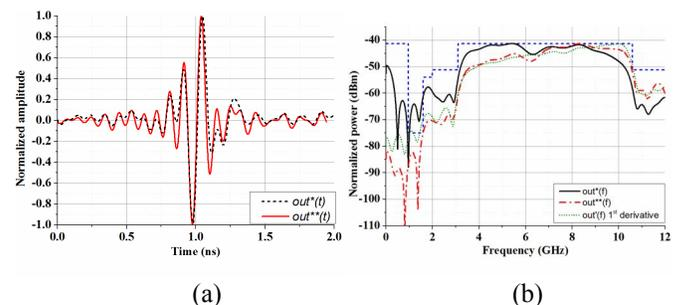
Figure 5: (a) Measured  $out^*(t)$  and post processed received pulse  $out^{**}(t)$  and (b) their normalized energy distribution versus the reference signal 1<sup>st</sup> order derivative.
