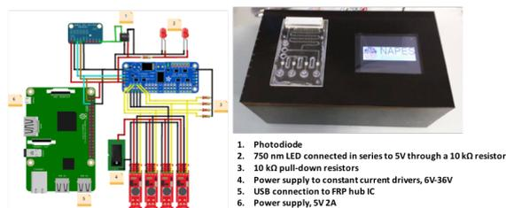
Figure 5: Detection and actuation platform showing the wiring diagram used and the final design including a touchscreen interface.
