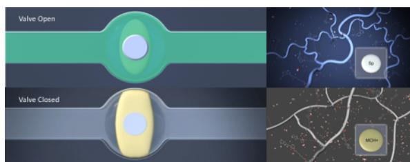
Figure 1: Hydrogel valves within microfluidic fluidic channels under light irradiation (open) and in the fully swollen (closed) states.
