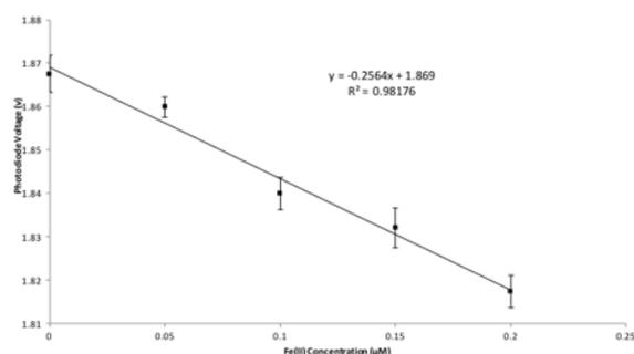
Figure 7: Calibration curve showing on-chip determination of Fe(II) concentration.
