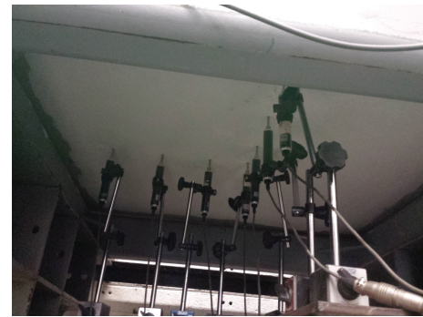
FIGURE 9: LVDTs positioned on the soffit of each slab.
