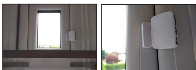
Figure 13. Contact sensor recording window opening.
