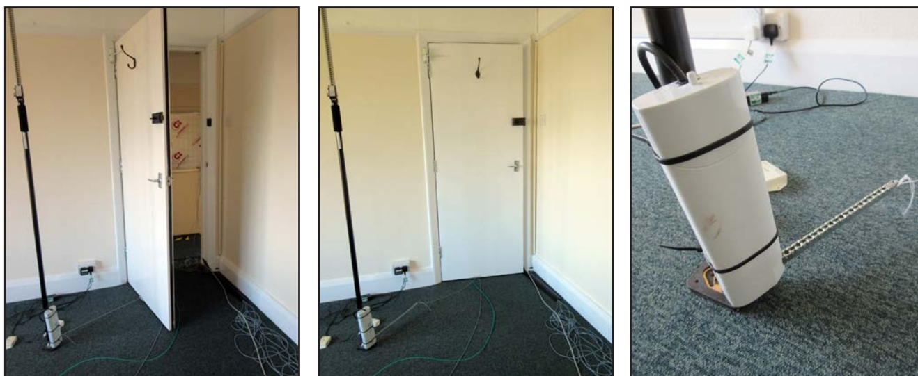
Figure 12. Internal doors controlled by a chain actuator.
