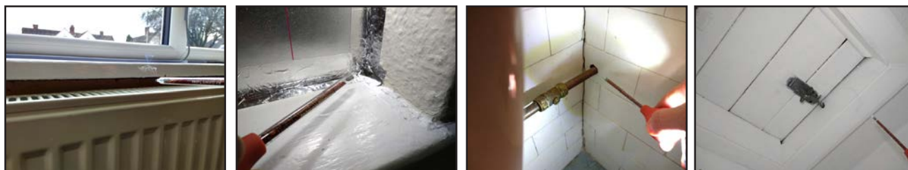
Figure 7. Qualitative air leakage testing using smoke sticks.
