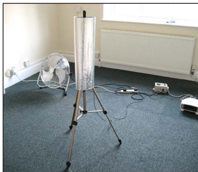
Figure 6. Co-heating equipment deployed in each room.
