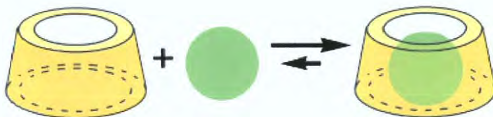
Figure 3. Formation of the inclusion complex of cyclodextrin with a small guest molecule. 18
