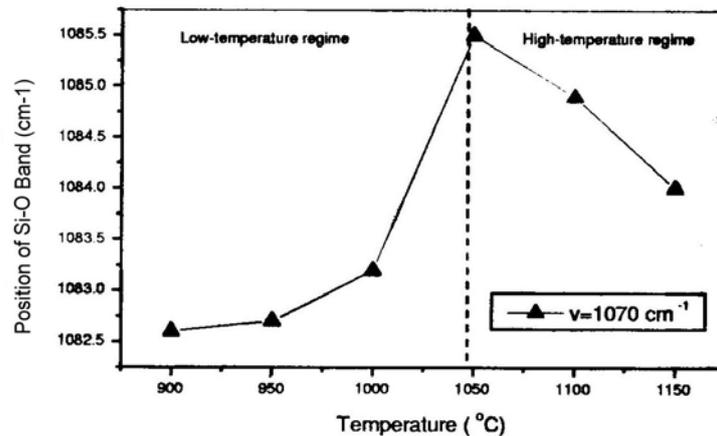
**Figure 2.** Peak position of the 1070cm<sup>-1</sup> band versus temperature
