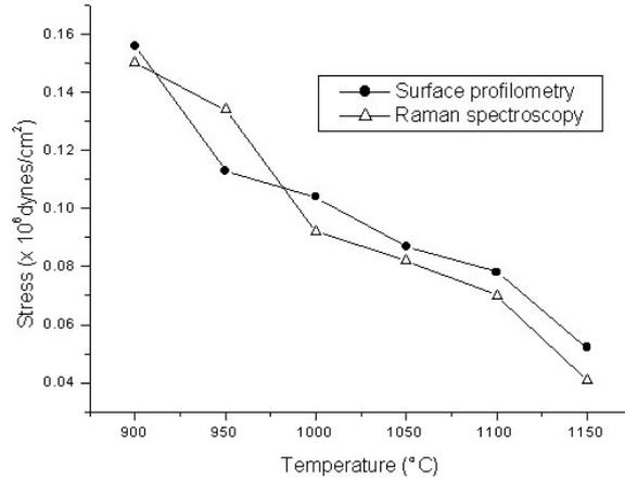
**Figure 1.** Wet oxide stress measurements
