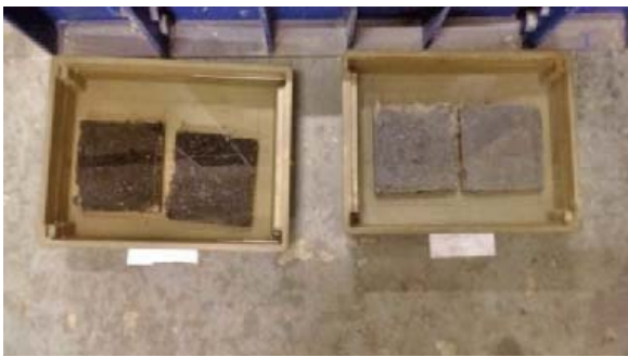
(b) Batteries stored in water and Epsom salt
