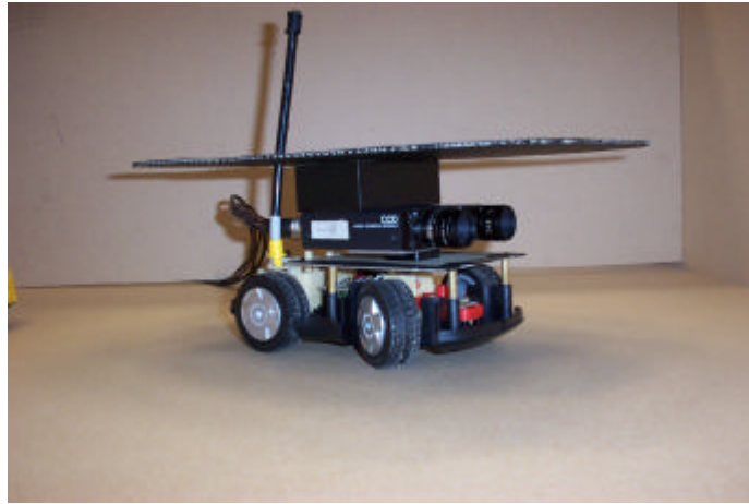
Figure 1 Mobile remote controlled stereo vision unit
