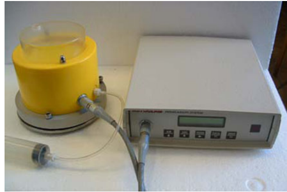
Fig. 4 Autoclam permeability apparatus [14]
