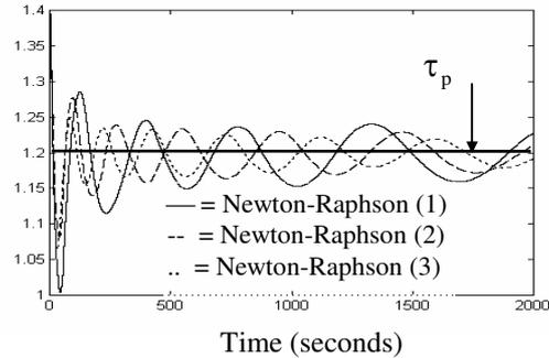
The figures show that the algorithms facilitate a reduction in mismatch between the process time delay and the model time delay.
