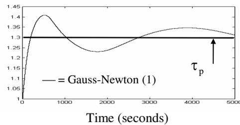
Case 3:  $G_m e^{-st_m} = 2e^{-s}/(1 + 18s + 137s^2 + 567s^3 + 1403s^4 + 2103s^5 + 1846s^6 + 856s^7 + 158s^8)$ ,  $G_c = 2.14(1 + 1/9.75s + 3.31s/(1 + 0.61s))$ .  $G_p = G_m$ .
