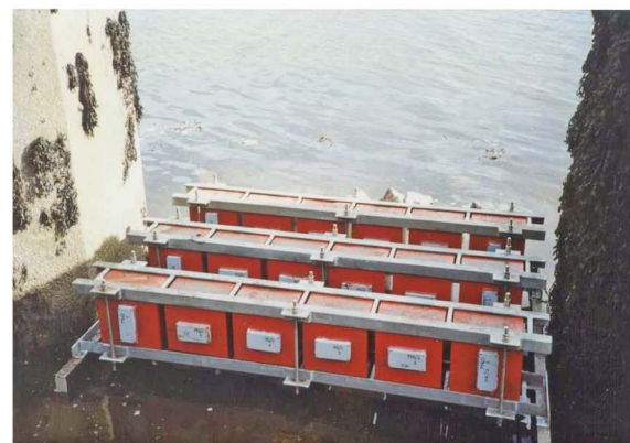
Fig. 3. (a) Location of marine exposure site; (b) slabs secured in galvanized steel frames showing the GRP enclosures
