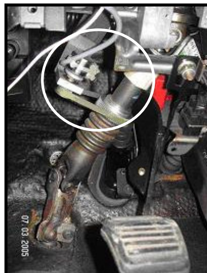
Figure 10: Rotary Potentiometer (circled) for sensing steering angle
