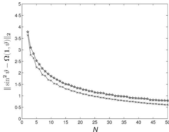
**Fig. 5** The norm of the residual for the swirl function with an increasing number of basis functions. The lower curve plotted with crosses is for Shankar's method while the curve plotted with stars shows Hills's collocation scheme
