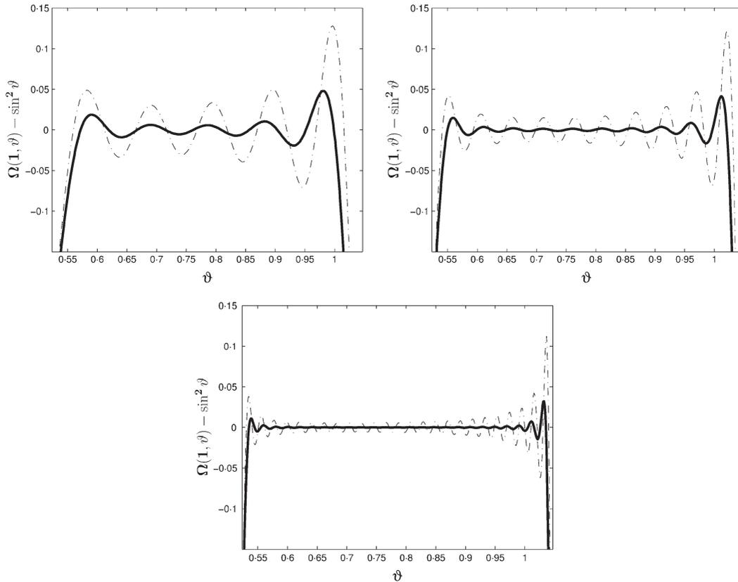
**Fig. 6** The residual at each point on the lid for the swirl function for  $N = 10, 20, 50$ . The dash-dotted line shows the residual for Shankar's method while the thick solid line shows residual for Hills's collocation scheme
