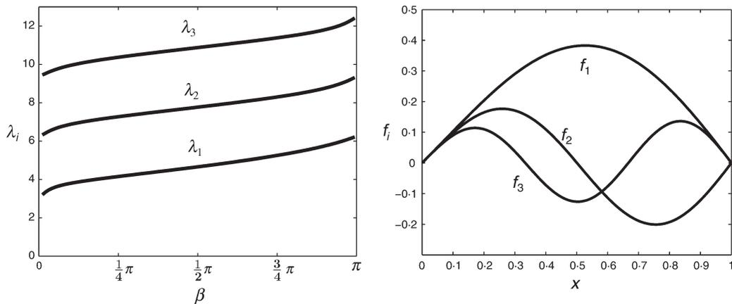
**Fig. 2** The plot to the left shows the first three (real) eigenvalues  $\lambda_i$  plotted against the outer angle  $\beta$  for a fixed inner angle,  $\alpha = 1^\circ$ . To the right are plotted the three first eigenfunctions  $f_i(x)$  for  $\alpha = 30^\circ$  and  $\beta = 60^\circ$
