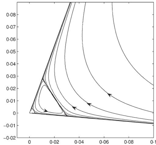
**Fig. 13** Eddies induced by the rotation of the outer cone since for  $\alpha = 20^\circ$ ,  $\beta = 95^\circ$ , the most slowly decaying mode is actually an eigenmode with  $\bar{\eta}_1 \simeq 4.89 + 1.35i$  and not a forced mode
