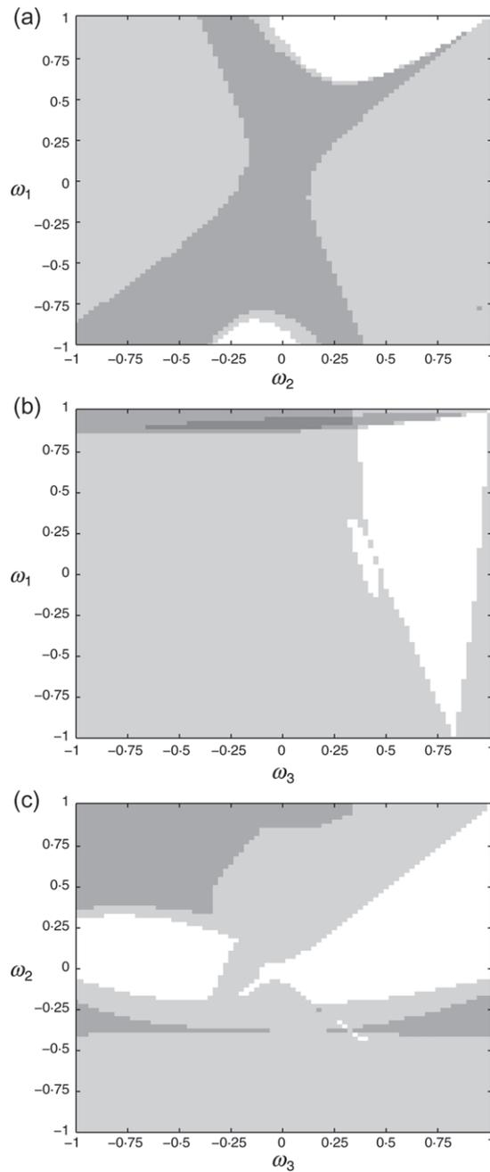
**Fig. 16** The number of circulatory regions present in the meridional stream function as a function of (a)  $(\omega_1, \omega_2)$  for  $\omega_3 = 1$ , (b)  $(\omega_1, \omega_3)$  for  $\omega_2 = 1$ , (c)  $(\omega_2, \omega_3)$  for  $\omega_1 = 1$ . The cone geometry is given by  $\alpha = 20^\circ$  and  $\beta = 75^\circ$  and the number of eddies is plotted by pixels varying from white (one eddy) to black (four eddies)
