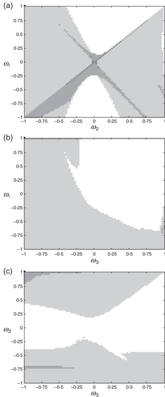
**Fig. 15** The number of circulatory regions present in the meridional stream function as a function of (a)  $(\omega_1, \omega_2)$  for  $\omega_3 = 1$ , (b)  $(\omega_1, \omega_3)$  for  $\omega_2 = 1$ , (c)  $(\omega_2, \omega_3)$  for  $\omega_1 = 1$ . The cone geometry is given by  $\alpha = 30^\circ$  and  $\beta = 60^\circ$  and the number of eddies is plotted by pixels varying from white (one eddy) to black (four eddies)
