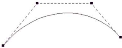
Fig. (9) Bézier curve with 4 control points [9]
