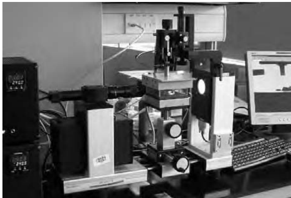
Figure 6. Overview of the complete test apparatus for measuring contact angles
