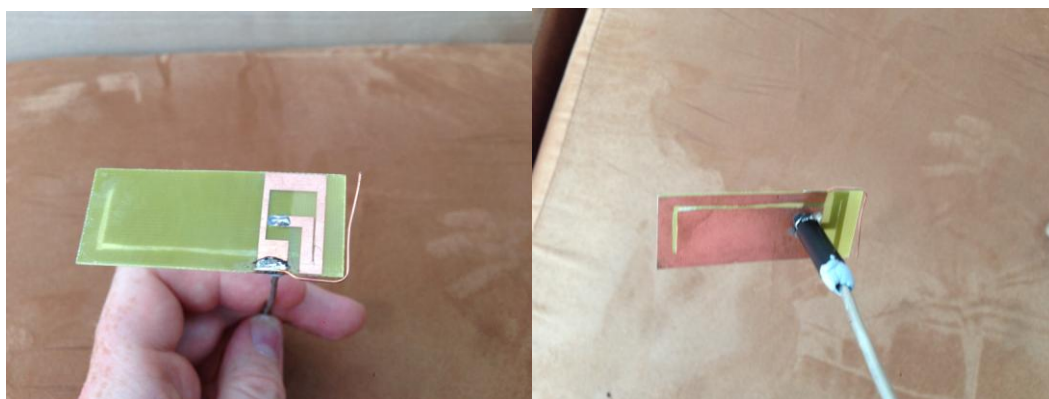
Figure 32: The empirical modifications made to the monopole side (left) and ground plane side (right) of the V50 prototype.
