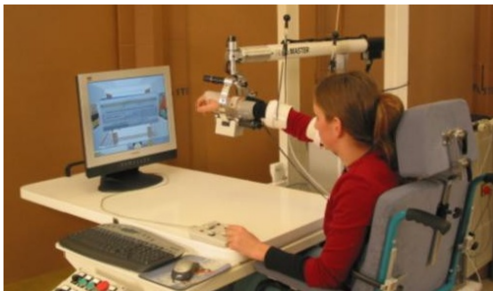
Figure 2-3: A person using the Gentle/s robotic rehabilitation system. Figure taken from [74].
