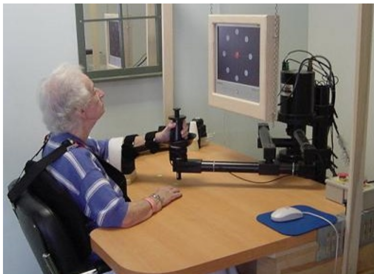
Figure 2-2: A person using the MIT Manus shoulder and elbow rehabilitation robot. Figure taken from [72].
