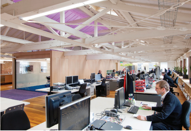
Figure 1. An open-plan office space, with separate enclosed meeting rooms, lit by a combination of electric lighting and daylight. The lighting distribution is unrelated to either visual tasks or the horizontal working plane, but is instead arranged to provide for a comfortable and pleasant working environment.
