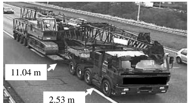
(b) GVW=100.8 t, wheelbase=22.3 m
