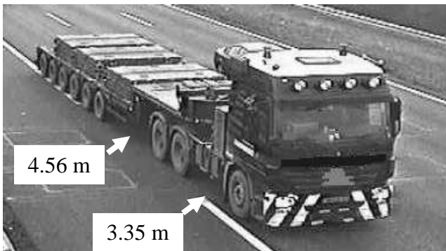
(a) GVW=100.1 t, wheelbase=16.2 m (carrying crane ballast).
