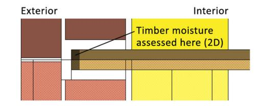
18 variations of a built-in joist end detail (using WUFI 2D) to check risk of timber decay at built-in joist ends
