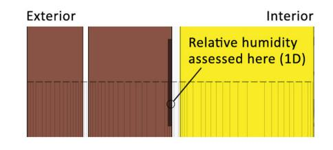
48 variations of a solid brick wall build-up (using WUFI Pro) to check risk of mould growth on original substrate
