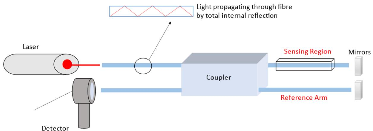
**Figure 5.** Operating principle of a transmission an interferometric fiber optic sensor. Light propagates through the optical fiber by total internal reflection. One arm of the coupler acts as a reference while the other is the sensing arm. The propagation of light in the reference arm is modulated by the presence of the analyte which changes the interference signal received by the detector.
