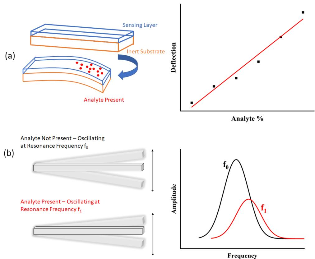
**Figure 2.** Cantilevers can operate in (a) static or (b) dynamic mode. In static mode, the cantilever bends due to a differential stress induced between the layers in the presence of the analyte. This deflection is measured as the means of sensing. In dynamic mode, the cantilever, magnetically or electrically actuated, oscillates at its natural frequency, but in the presence of the analyte the resonance frequency changes.
