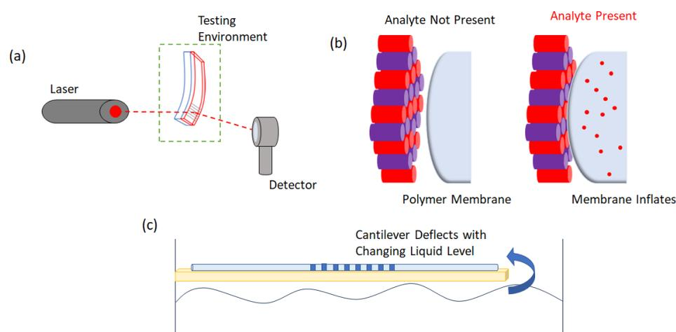
**Figure 8.** Operating principle of several diffractive optomechanical sensors. (a) Static deflection cantilever sensor combined with a diffraction grating. This is similar to the sensor presented by Grogan et al. [110] where diffraction efficiency of the grating changes depending on the angle of deflection of the cantilever
