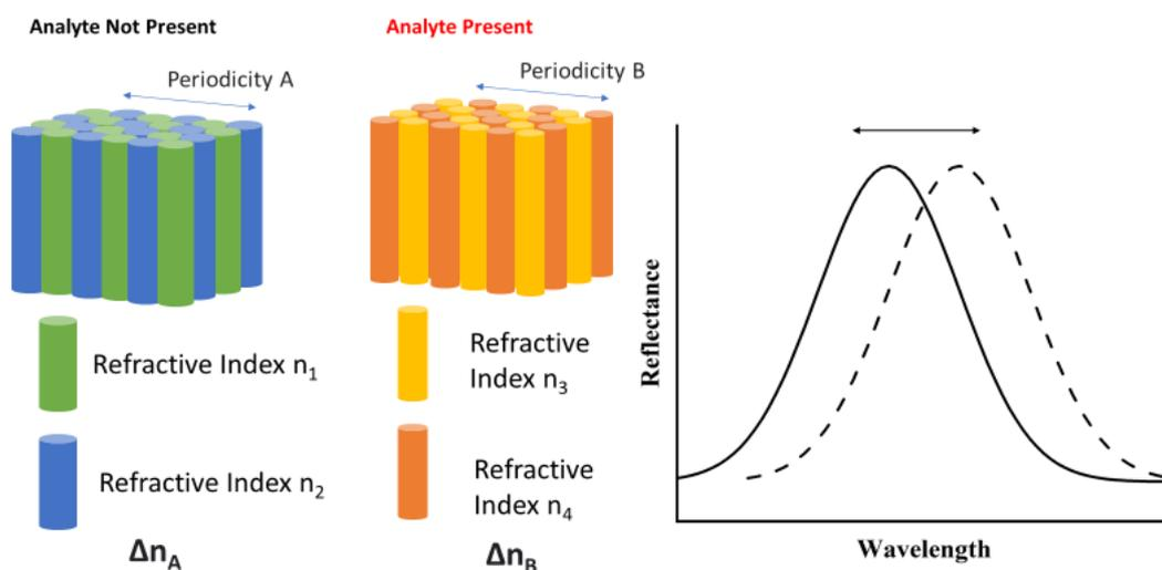
**Figure 7.** Operating principle of a 2D Photonic Crystal Sensor. The presence of the analyte causes a change in the refractive index modulation and/or the periodicity of the crystal. This results in a shift in the peak wavelength of reflected light.
