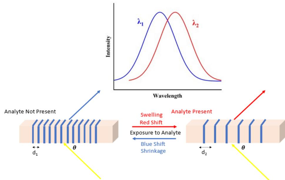
**Figure 4.** Operating principle of a transmission holographic sensor (where  $d$  is the grating spacing and  $\theta$  is the angle of the incident beam on the grating). In this particular sensor configuration, when the analyte is present, the grating spacing changes leading to a change in the peak diffracted wavelength and the intensity of the diffracted beam.
