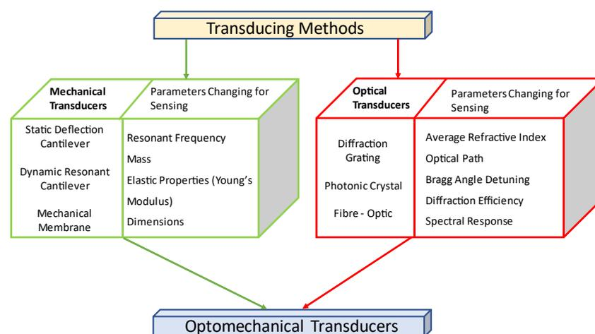
**Figure 1.** Foundations of optomechanical sensors. The typical response and parameters used by such sensors are presented, various combination being implemented.
