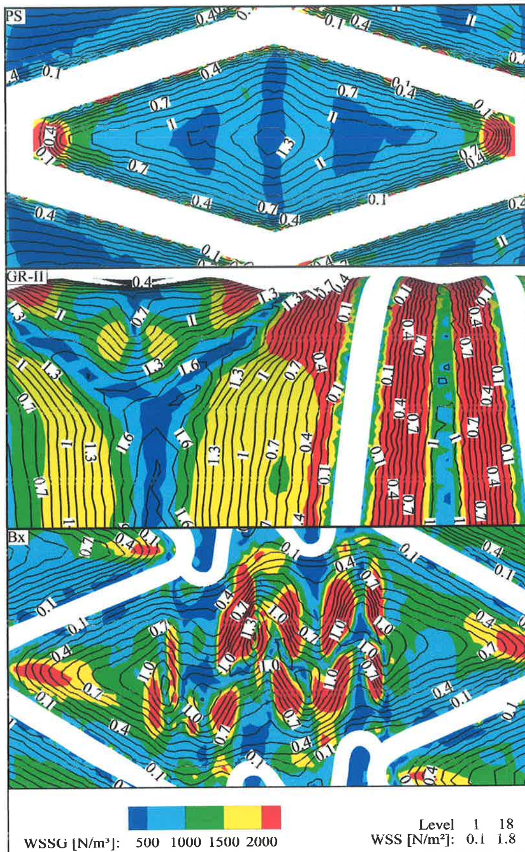
Figure 6-22: Contour plots of WSSG near the PS, GR-II and Bx stent struts with overlaid line contour plots of WSS (labelled by magnitude [ \text{N}/\text{m}^2 ]).
