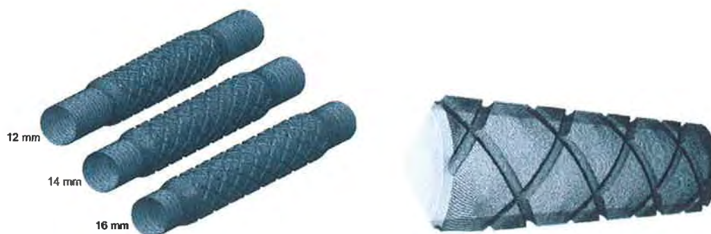
Figure 4-1: (A) Three models of a stented coronary artery which are different lengths due to foreshortening from LaDisa et al. [62]. (B) Model of a stented coronary artery from Rajamohan et al. [99].
