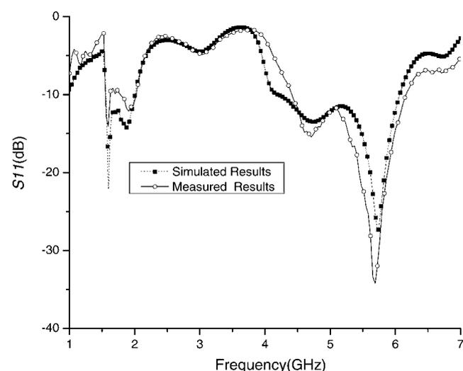
**Figure 8** Comparison of the simulated and measured  $S_{11}$  for Antenna A
