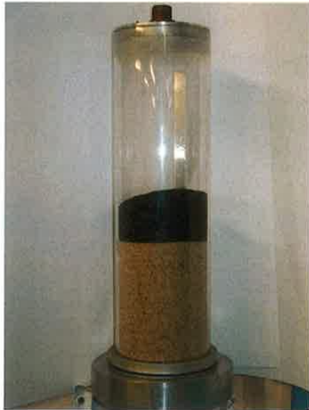
Figure 2.25. Multi Media Filter at Rest.
