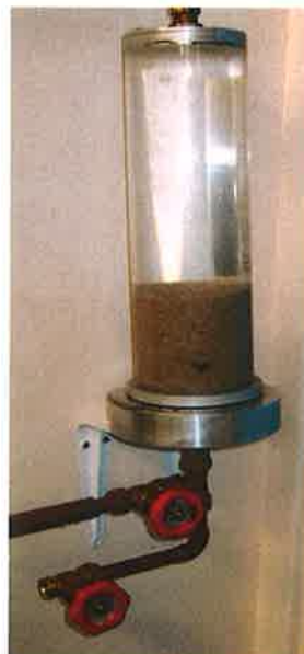
Figure 3.19. Filter at Rest.
