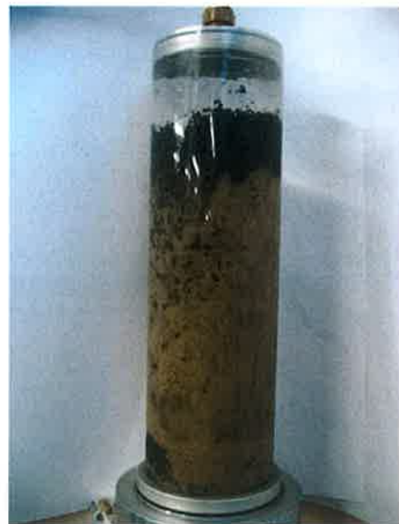
Figure 2.26. The Filter During the Backwash Cycle,
