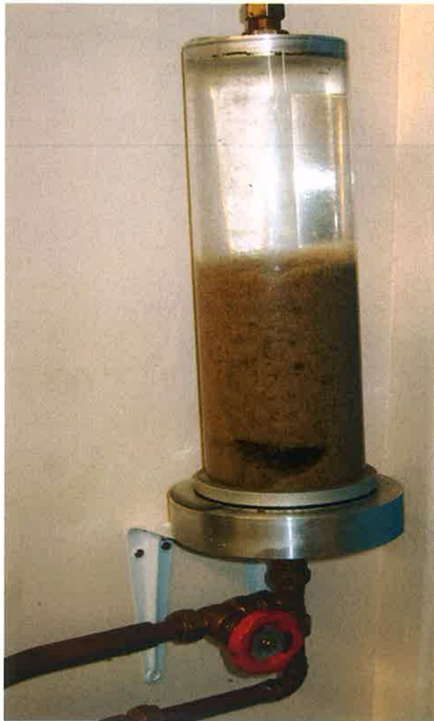
Figure 3.20. Filter Bed Expanded During a Backwash Cycle.
