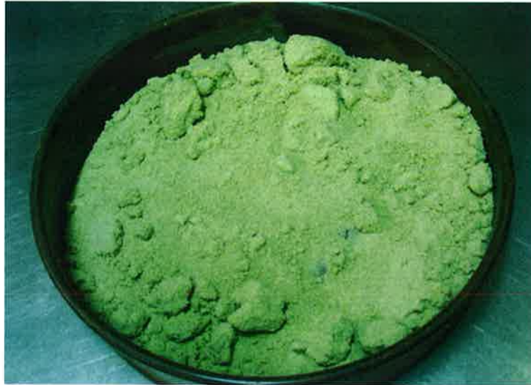
Figure 3.5. Sand Sample after Drying, Ready for Grading.
