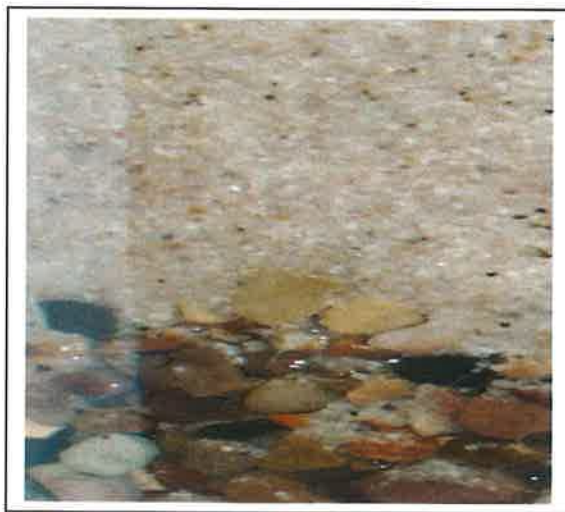
Figure 3.14. The Effects of the Fines in the Sand on the Support Gravel.
