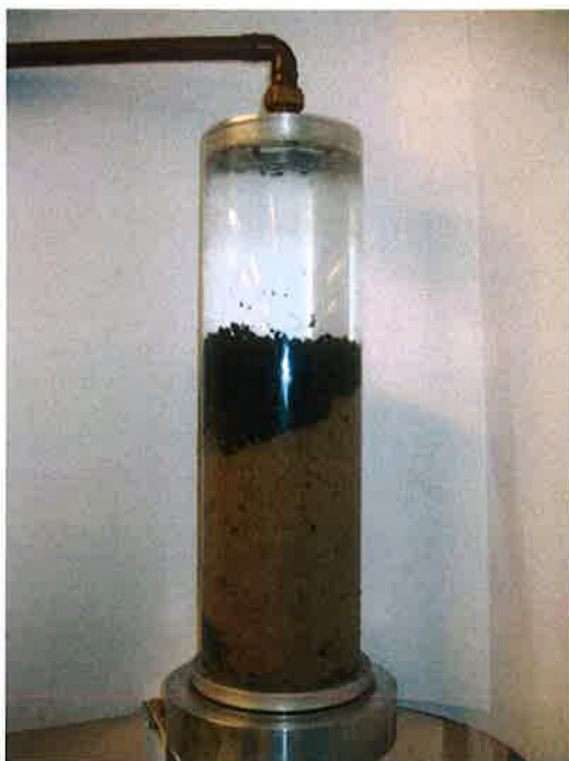
Figure 2.27. The Filter at Rest after Backwashing.
