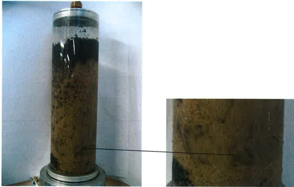
Enlarged View of the Swirling Action During Backwash.
