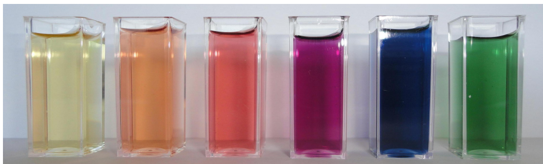
Figure 1. A sample set of the different coloured Silver colloids produced in the practical.
