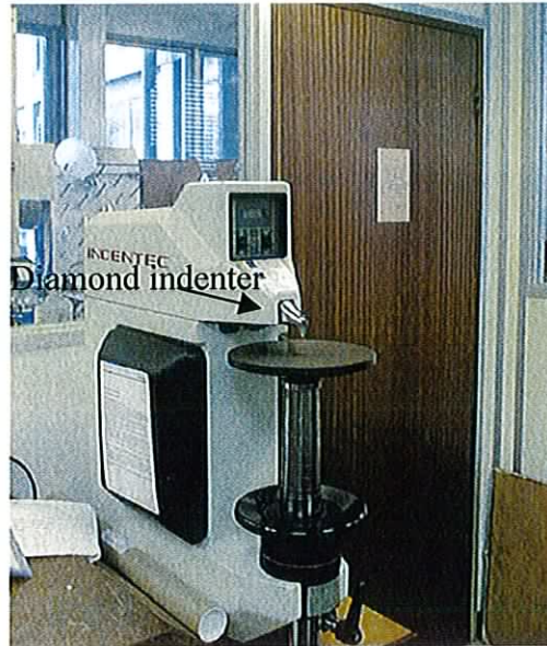
Figure 2.5: The Rockwell indentation tester. The diamond indenter lies above the sample holder. The load increases on the diamond creating an indent in the coating and substrate. The indent can be analysed for cracks.
