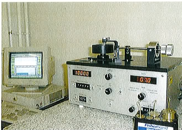
Figure 2.15: A photograph of a pin-on-disk wear tester. The balancing arm with the pin attached to it can be seen to rest on the sample to measure the friction coefficient of the coating.
