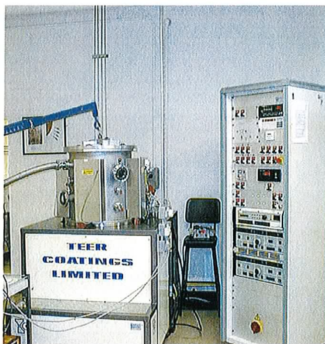
Figure 3.1: Closed field unbalanced magnetron sputtering system. On the right of the photograph is the rack cabinet which controls the DC power supplies, gas flow rates, optical emission monitor, pumping system, pressure gauges and valves. On the left of the photograph is the chamber which houses the four magnetrons and the pumping system below the chamber. There is also a hoist attached to the chamber lid. The portholes on the chamber can be used to view the plasma and substrate during deposition.
