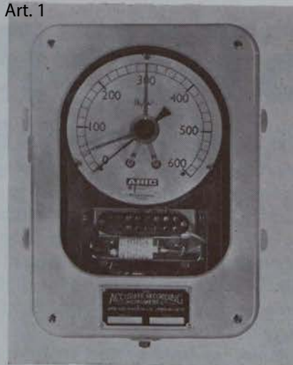
One of the ARIC indicating pressure controllers. (See report).
