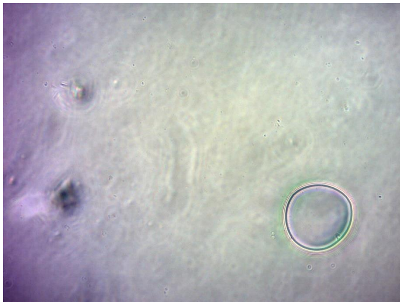
Figure 9: Image captured of sample run on microfluidic device for liposome synthesis, viewed on an inverted microscope at 400X total magnification
