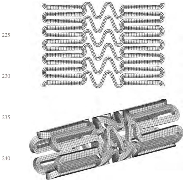
Figure 1. 'Wrapping' of planar stent geometry (top) into its cylindrical configuration (bottom).
