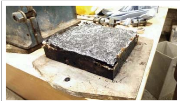
(a) Layered cement-based battery
