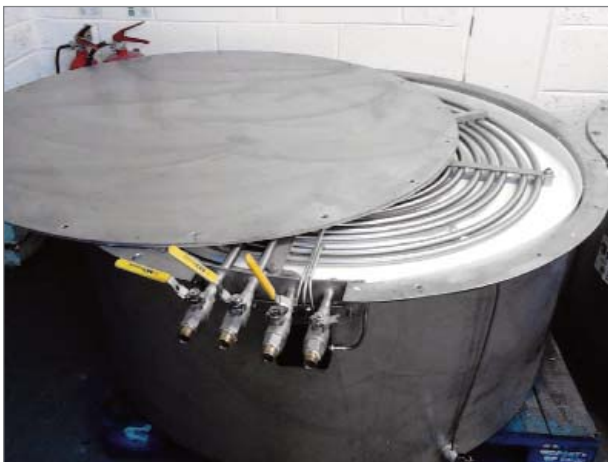
Figure 1: Prototype 500-litre PCM-TES unit.
