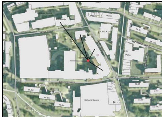
Fig. 10. Identifying buildings using directional query vectors
