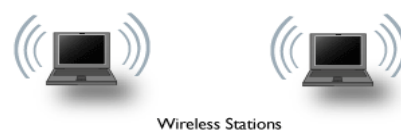
Figure 2.2 (b): Basic Service Set ( ad-hoc ).
