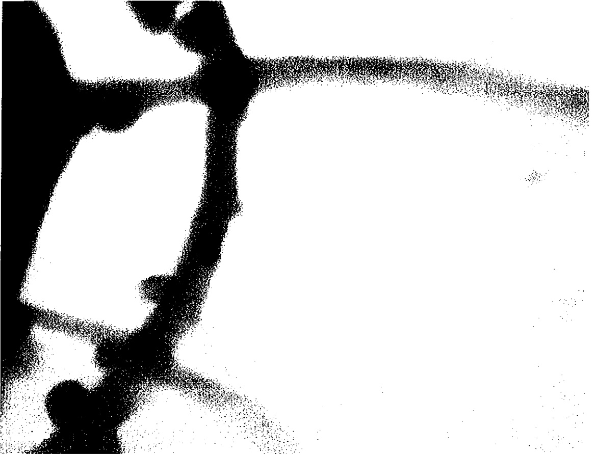
Figure 2 TEM images of untreated H-SWNT at a magnification of 100,000X. The bundle-like structures represent the SWNT bundles and the circular structures represent the iron catalyst particles.
