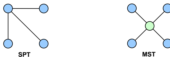
Figure 2-14: Four nodes connected using a SPT. MST connects the same four nodes by placing an additional Steiner node.
