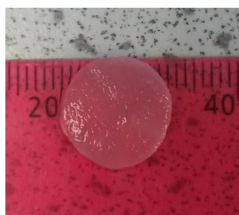
Figure 4. Tensile testing and compressive testing shows when fibrin gels are supported with a 0.75%Collagen 0.044%GAG matrix, their mechanical properties change significantly.
