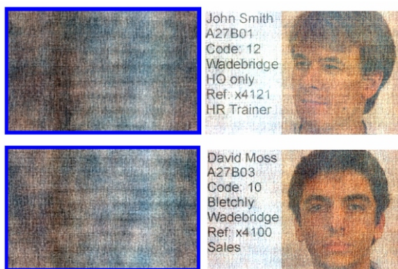
Figure 7. Composite images that include a (blue) reference frame for automatic cropping and orientation. In each case, the data fields (left hand side) have been printed and scanned at 300 dpi. The reconstructions on the right-hand side are the outputs obtained after re-sizing the scanned data to the size of the noise field used for encrypting the original images and then correlating the (re-sized) data with the noise field.
