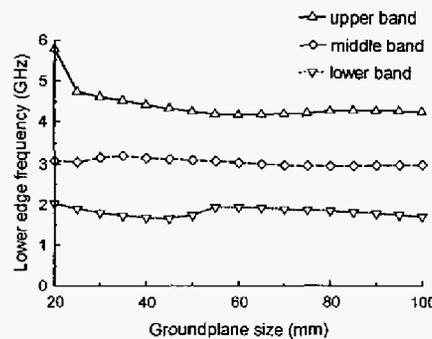
Figure 5. Lower edge frequency dependence on groundplane size
