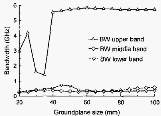
Figure 4. Impedance bandwidth dependence on groundplane size
