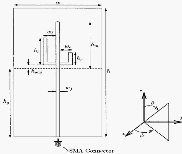
Figure 1: Geometry of the printed multibranch monopole
