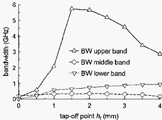
Figure 3. Impedance bandwidth dependence on tap-off point
