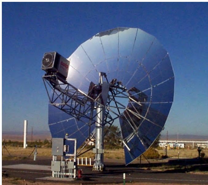
Figure 2.6 Solar Dish / Stirling system [66]
