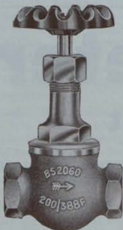
Renewable Disc Wheelvalve BS 2060 — Class 200 W.P. 200 PSI at 388°F.
