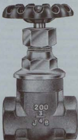
Gunmetal Gatevalve BS 1952 — Class 200 W.P. 200 PSI at 388°F.
