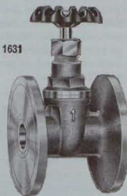
Flanged Gunmetal Gatevalve Spindle dia. & Face to Face to BS 1952 Class 200 W.P. 150 PSI at 366°F.
