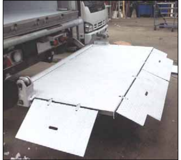
Figure 4.27. Photograph of tail-lift showing the coating applied to the mild steel platform
