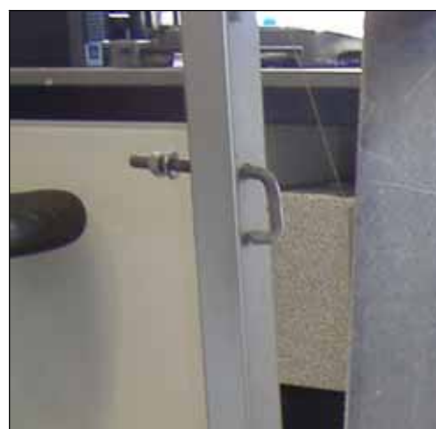
Figure 4.22. Photograph showing the clamp which comprises a threaded shaped rod to clasp the holding frames and the panel together.
