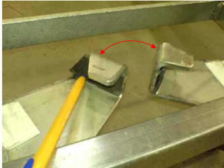
Figure 5.7. Photograph of rubber stoppers fitted to the inside surfaces of the base frame to reduce the noise of the impacting A-frame during folding.
