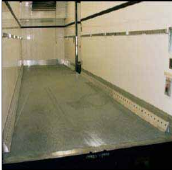
Figure 4.26. Photograph of the inside of a HGV trailer showing uncoated chequered aluminium flooring.
