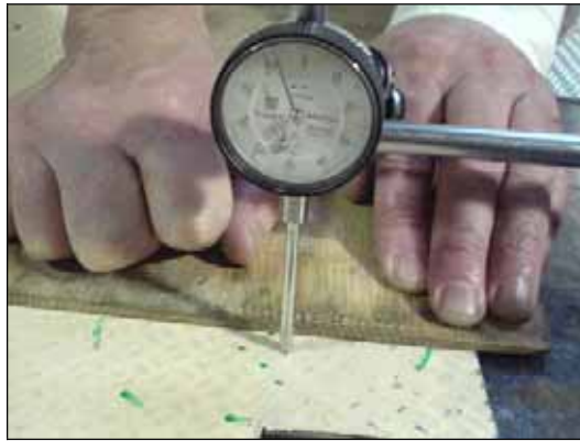
Figure II.3. Photograph showing a measuring point on an abraded part of panel A.
