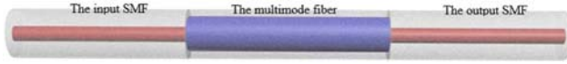
FIGURE 1 Schematic of SMS fiber structure [Color figure can be viewed at wileyonlinelibrary.com]
