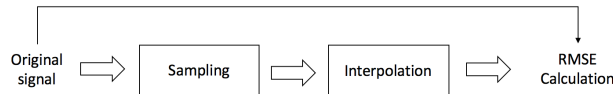
Fig. 4. The methodology to calculate the best interpolation method is based on the RMSE between the original signal and the reconstructed one.
