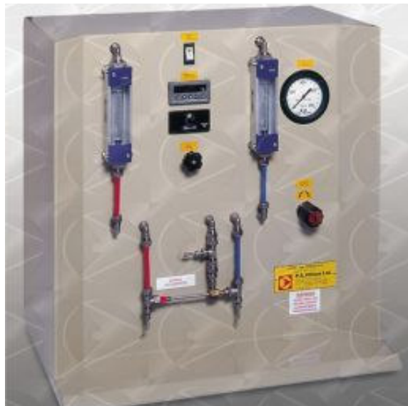
Fig. 1-12: Experimental RHVT Equipment, by P.A. Hilton Ltd [14].
