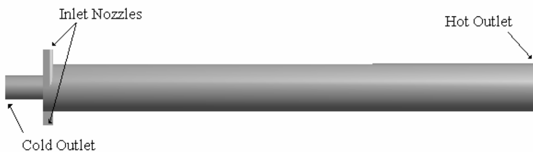
Fig. 4-3: Plan view of the CFD model of the 3D RHVT with two inlet nozzles, cold outlet and a conical hot outlet.
