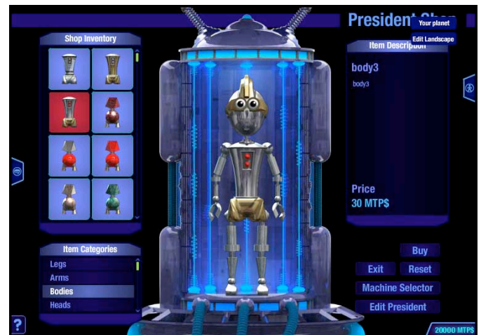
Figure 4: Runtime asset selection during user configuration. The user is provided with a list of possible body parts taken from the 8 available robot characters. When a selection is made the avatar skeleton is updated by loading in that asset, while also triggering an interaction phrase (section 3) relating to the body part.
