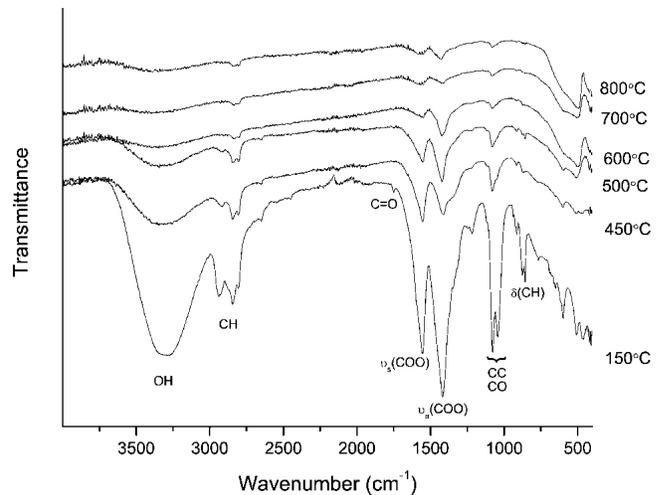
FIG. 6. FTIR spectra of Pb<sub>0.5</sub>Ba<sub>0.5</sub>TiO<sub>3</sub> powders with varied calcination temperatures ( $T_c = 150, 450, 500, 600, 700, 800$  °C).
