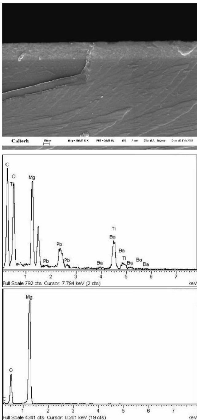
FIG. 7. Cross-sectional analysis of  $\text{Pb}_{0.5}\text{Ba}_{0.5}\text{TiO}_3$  thin film: (a) FE-SEM, (b) EDX of film, and (c) EDX of substrate (note: cross section was coated in carbon for enhanced detail).
