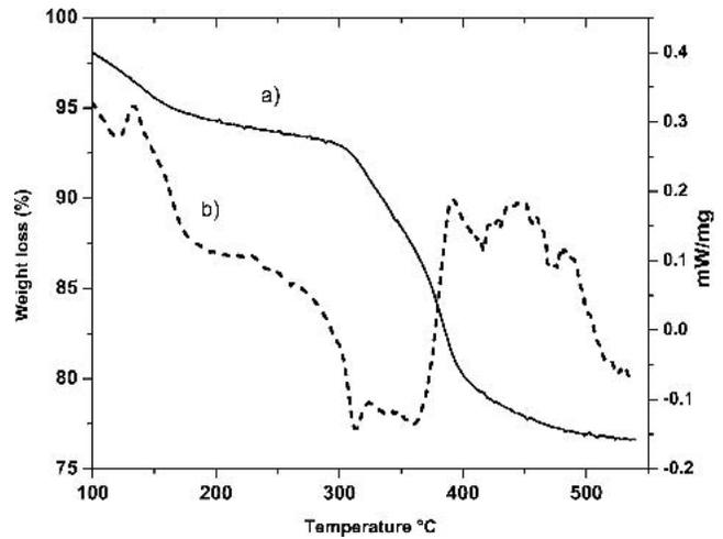
FIG. 5. (a) TGA and (b) DSC curves obtained from a Pb<sub>0.5</sub>Ba<sub>0.5</sub>TiO<sub>3</sub> powder sample prepared with  $R_w = 8$  and  $R_A = 4$ .
