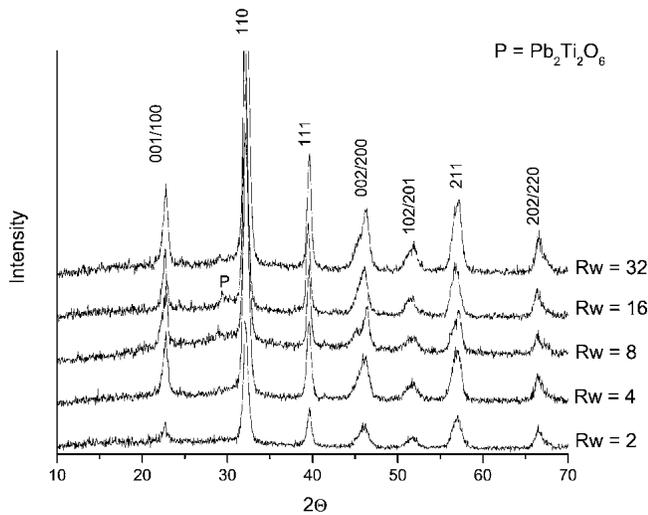
FIG. 3. X-ray diffraction patterns obtained from Pb<sub>0.5</sub>Ba<sub>0.5</sub>TiO<sub>3</sub> powder samples with  $R_w$  values as indicated (calcined at 600 °C, 2 h).
