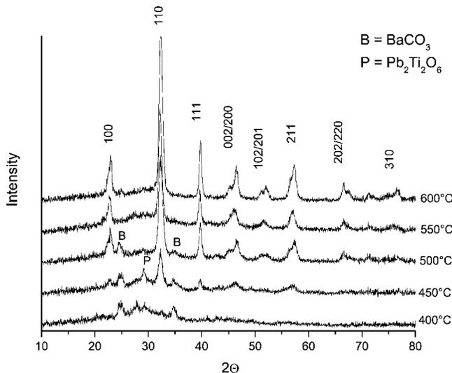
FIG. 4. X-ray diffraction patterns obtained from Pb<sub>0.5</sub>Ba<sub>0.5</sub>TiO<sub>3</sub> powder samples calcined at the temperatures indicated ( $R_w = 8$ ,  $R_A = 4$ ).
