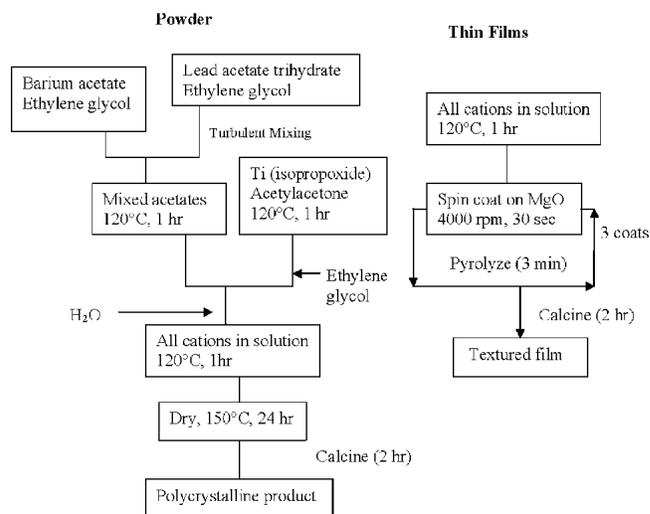
FIG. 2. Sol-gel synthesis of powder and thin film Pb<sub>0.5</sub>Ba<sub>0.5</sub>TiO<sub>3</sub>.
